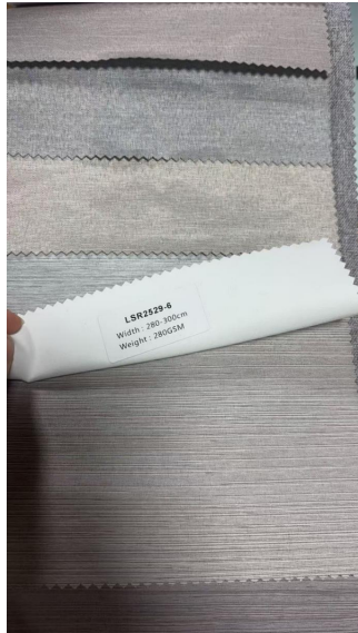
LSR2529 technology: double composite composition: 100%polyster width: 300cm weight: 270g
